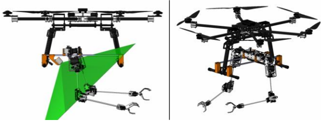
Figure 3. 3D view of the arms integrated in the hexarotor platform between the legs of the landing gear. A ZED camera provides 120 deg FoV (green).
